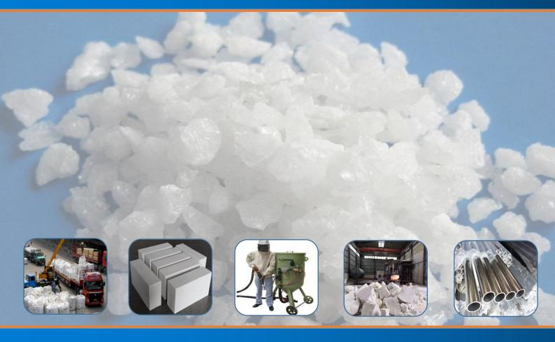
White Fused Alumina (WFA, WA) is a synthetic corundum made of reduced fusion of high purity alumina powder and other fillings in electric arc furnace under 2000 degrees above. Its main chemical content is Al2O3(99% min), little Na2O, Fe2O3 and SiO2.
