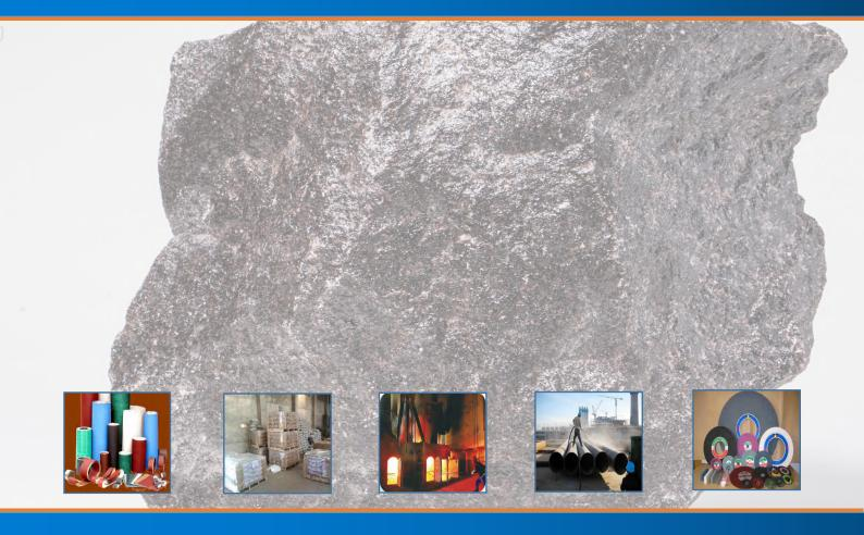
Brown Fused Alumina is an important synthetic corundum refractory mineral made from reduced fusion of quality bauxite iron and coal in electric arc furnace under 2500 degrees.
